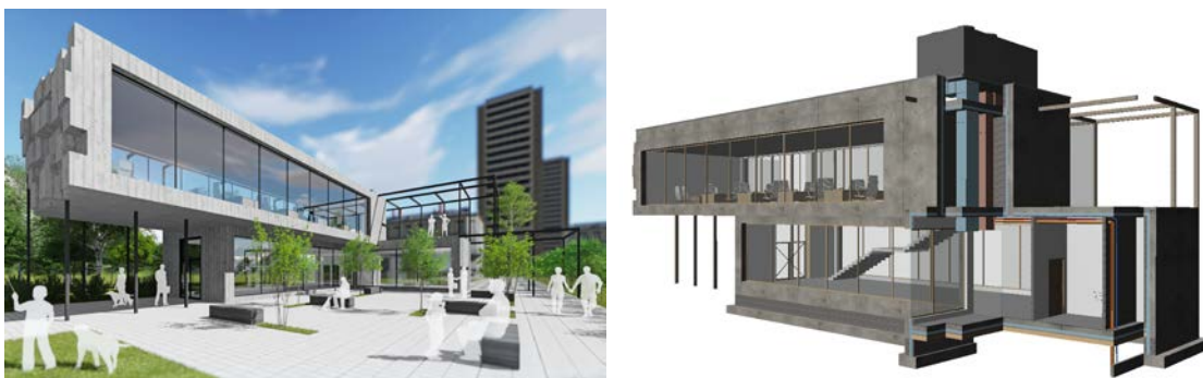
Figure 3: Student's work - exhibition pavilion with reading room. Load-bearing functions were assigned to elements to generate the structural framework (Author: Yaroslav Matvieiev, 2018).
