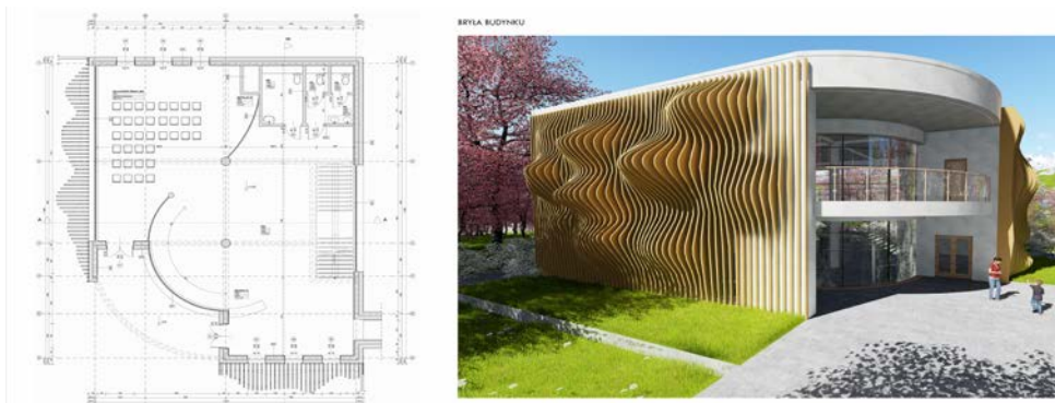
Figure 2: Student's work - exhibition pavilion with reading room. Example of creating the details and profile walls, which is necessary to generate advanced cross-sections and system solutions (Author: Julia Sierpień, 2018).
